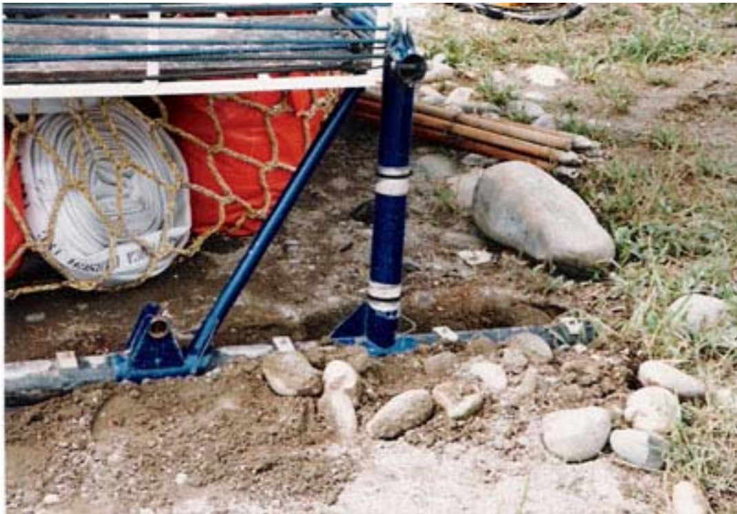
Skid sunk into ground from impact
